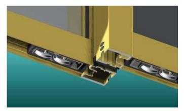
Series 702 SlideMASTER™ panels are fitted with heavy duty double bogey wheels as standard. The wheels are matched to the diameter of the sill running rails. The result is smooth silent running door panels.
