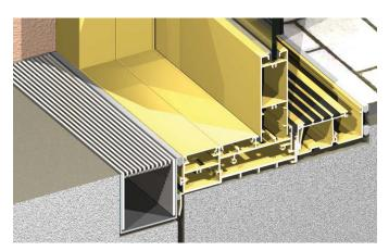
The illustration above shows the fully recessed sill with Centor SI roller screen on the inside and a recess sump on the outside. This is the ultimate building-in detail.
