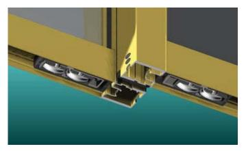
Series 704 SlideMASTER™ panels are fitted with heavy duty double bogey wheels as standard. The wheels are matched to the diameter of the sill running rails. The result is smooth silent running door panels.
